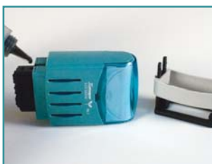
Remove the Impression Frame™ and use an ink cartridge to put 2-3 drops of ink into the inking hole. Put 2-3 drops into the frame as well.
